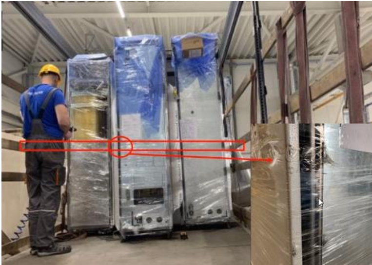
Figure 5 Risk of damage by stretching frames
