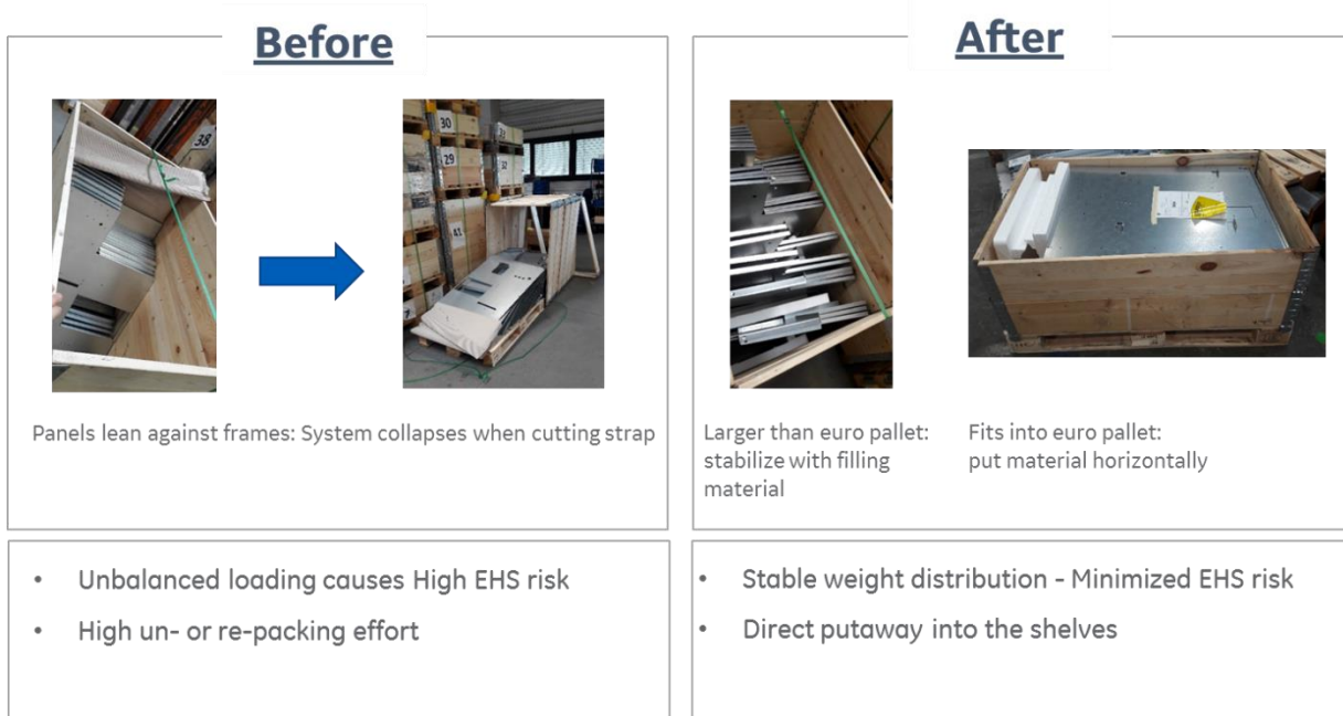
Figure 9 Dangers of loading units of large sheet metal parts
