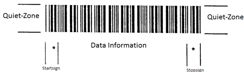
Figure 14 Barcode with Quiet-Zones and Start-/Stop sign
