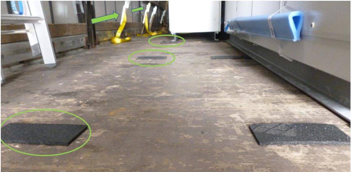
Figure 4 Usage of anti-slip mat under skid frame as additional transport protection
